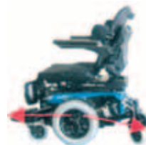
Groove M, MWD TR = Center of drive wheel to most distant point - tends to have shortest TR
